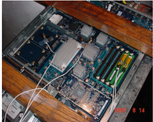
Fig. 6. Accelerometer locations on the unit
